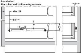
Gap width S = 12 to 15 mm Not self closing (without lowering) Y= 21 mm Self closing Y = 23 mm
