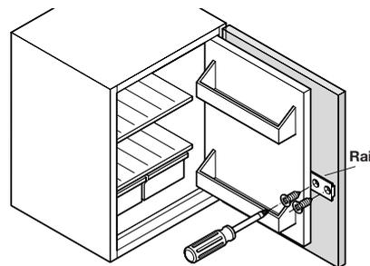
Open the refrigerator door by 90° and insert the rail into the guide (see "X" on plan drawing).
