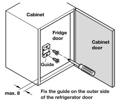
max. 8 Fix the guide on the outer side of the refrigerator door
