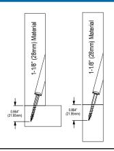
Material - Joining 1-1/4" (32mm) to 1-1/4" (32mm) Recommended screw length - 2" (51mm)
