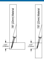
Material - Joining 1" (25mm) to 1" (25mm) Recommended screw length - 1-1/2" (38mm)
