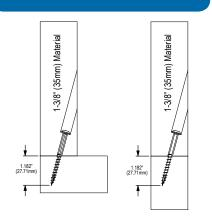
Material - Joining 1-1/2" (38mm) to 1-1/2" (38mm) Recommended screw length - 2-1/2" (63mm)
