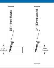
Material - Joining 1-1/8" (28mm) to 1-1/8" (28mm) Recommended screw length - 1-1/2" (38mm)
