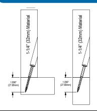
Material - Joining 7/8" (22mm) to 7/8" (22mm) Recommended screw length - 1-1/2" (38mm)
